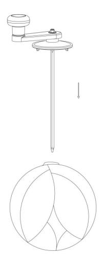
Assembly Step 7 Insert the core into the hole.
